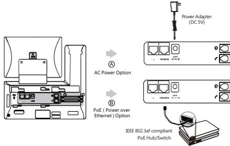
**Note:** The phone should be used with Yealink original power adapter (5V/2A) only. The use of the third-party power adapter may cause the damage to the phone.
