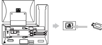
**Note:** The USB port can also be used to connect other USB devices, such as EXP50, USB headset and so on.
